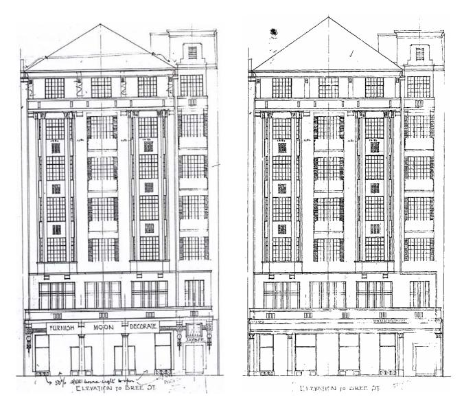
Top left and right: extracts from two different municipal submission drawings, showing the Bree Street elevation of the proposed building. Both drawings are dated March 1929. The drawing on the left was signed on 23 March 1929 and the one on the right, on 8 May 1929, by the City Engineer.. As no other elevation plan could be found, it remains difficult to confirm which of these elevation plans was eventually implemented.
